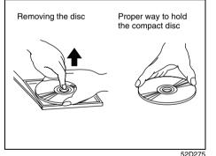
To remove a compact disc from its storage case, press down on the center of the case and lift the disc out, holding it carefully by the edges.
